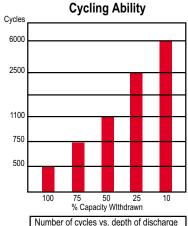
Number of cycles vs. depth of discharge at +20°C discharge with 20 hour rate
