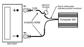
Figure 2. Direct Connection to Battery
